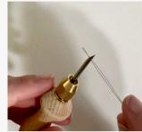
2. Put threading needle into the center hole of the needle and push thru the shaft to the other end of the needle (handle side.
